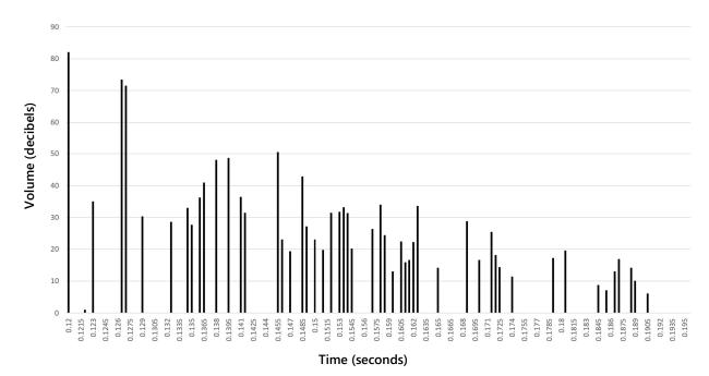
Reflectograms measure the amplitude, or volume, of sound over time. The vertical axis shows the volume (measured in decibels) of the recorded sound, while the horizontal axis shows the time (measured in seconds) for that sound to be picked up by the microphone.
